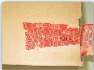
FIGURE 10 Security tape used for asphalt mix samples.
