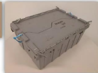
FIGURE 12 Tamper resistant security seal for asphalt pavement core sample cases.
