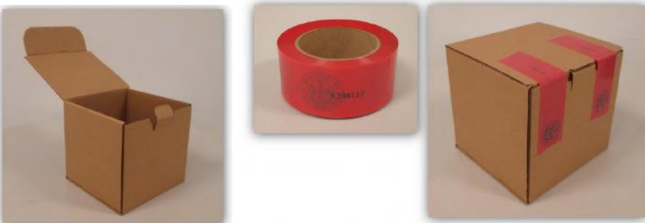
FIGURE 10 Security tape used for asphalt mix samples.
